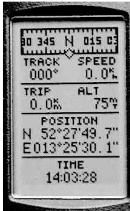
Fig. 7 Position page with position and altitude above mean sea level
