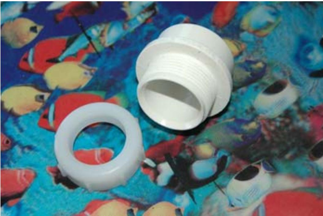
I also found what is called a 1 1/5" straight adapter that has a 1 1/2" male side and a female compression thread on the other side. I take that PVC adapter and spray paint it flat black. Then I take a sheet of 65# black card stock and cut two strips 3/4 inch wide and a total of 20.25 inches long (one 11" and one 9.25" strip) and I tightly wrap and scotch tape these to shim the male side of the PVC to fit snugly into the optical tube.
