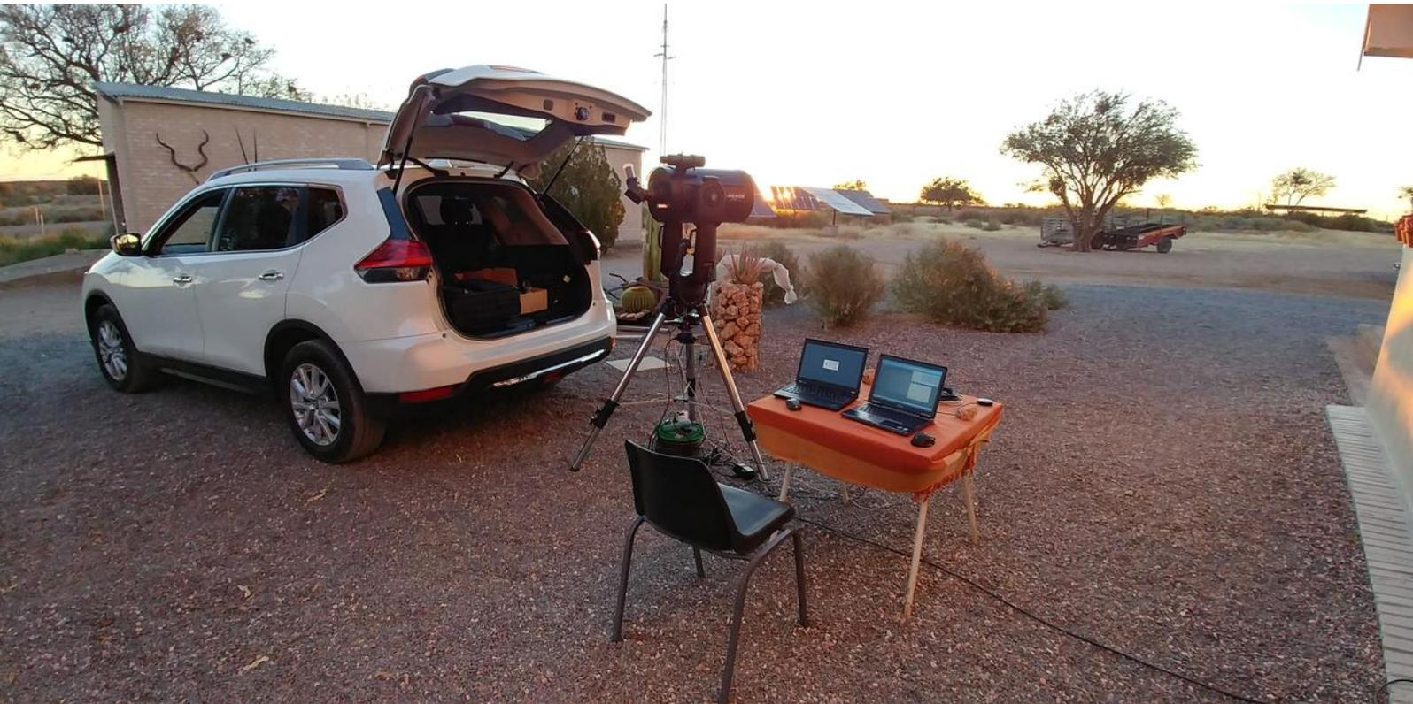
Figure 6. Set up of the instruments (Meade 10-inch LX90 + Raptor Photonics Merlin EM247 EMCCD camera), immediately after arriving at this site, where the sky started to clear up.
