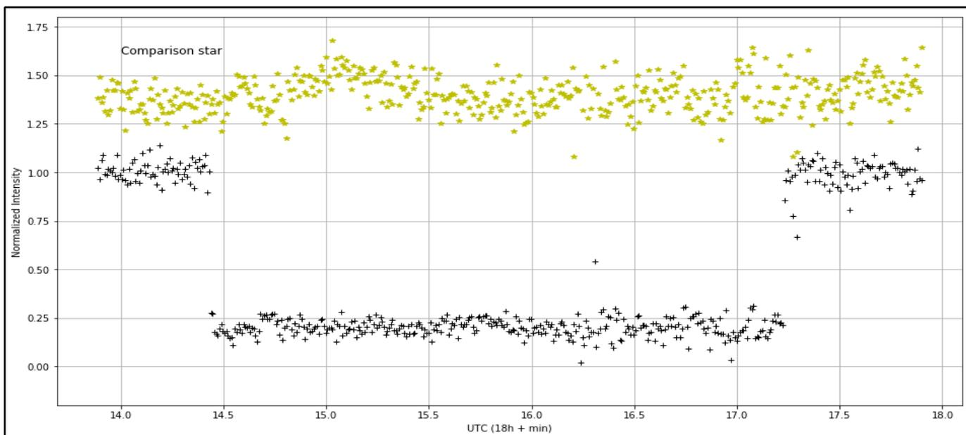
Figure 7. Occultation light curve acquired by the mobile station using a 0.254 m SCT + Raptor Photonics Merlin EM247 EMCCD camera. Exposure time was 0.5 s. Site location : lat 28 03 35.150 , lon 21 01 31.631 , alt 873 m. Observer: M. Kretlow. Due to wind and tracking problems the quality of the photometry decreases partly after about mid-occultation.
