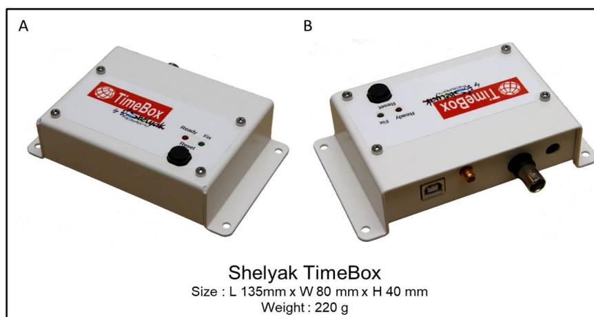
Figure 1. The Shelyak TimeBox, a device designed for accurate UTC time recordings with digital video cameras.
