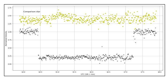
Figure 7. Occultation light curve acquired by the mobile station using a 0.254 m SCT + Raptor Photonics Merlin EM247 EMCCD camera. Exposure time was 0.5 s. Site location : lat 28 03 35.150 , lon 21 01 31.631 , alt 873 m. Observer: M. Kretlow. Due to wind and tracking problems the quality of the photometry decreases partly after about mid-occultation.
