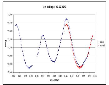
Figure 2. The brightness curve of Kalliope of February 12<sup>th</sup> 2017. On the x-axis the Julian date minus 2457797 and on the y-axis the V magnitude. The first part of the curve is copied on top of the second part of the curve, in red. The end of the eclipse is now easy to find, at about JD 0.51, but not the start of the eclipse because the first part of the curve cannot serve as a reference.
