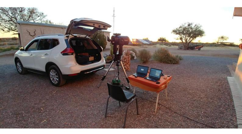
Figure 6. Set up of the instruments (Meade 10-inch LX90 + Raptor Photonics Merlin EM247 EMCCD camera), immediately after arriving at this site, where the sky started to clear up.
