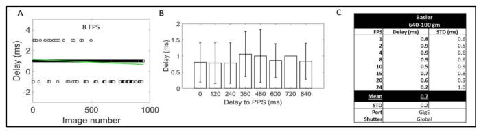
Figure 5A-C. Shelyak TimeBox in Trigger mode allows accurate millisecond timestamping of recordings with I/O triggered digital cameras. A I/O triggered Basler 640-100gm digital camera was used to record a SEXTA device for 2 minutes at different acquisition frequencies; the recording frames were triggered using a Shelyak TimeBox in Trigger mode at different frequencies. The recorded frames were captured using Airylab Genika as acquisition software.
