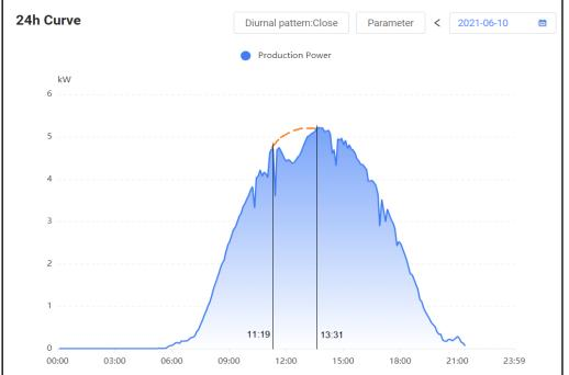
Figure 6. Partial eclipse clearly visible in power production curve of 2021 June 10.
