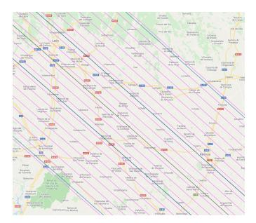
Figure 3. Zoomed detail of Marc Buie's prediction showing the 22 chords evenly distributed between both 3-sigma limits. Separation between chords was 4.7 km and each one was used to establish all the 22 observing stations. (Google Maps)
