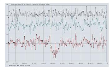
Figure 3. Light curve of the occultation by 2004  $XR_{190}$  on 2021 Jan 22, recorded by the author with a f/4 0.4 m Newtonian, a Mintron 12V6HC-EX camera, which was set to a frame rate of 6.25 fps, and a Kiwi time inserter. The star image stability was reported as bad to fair.
