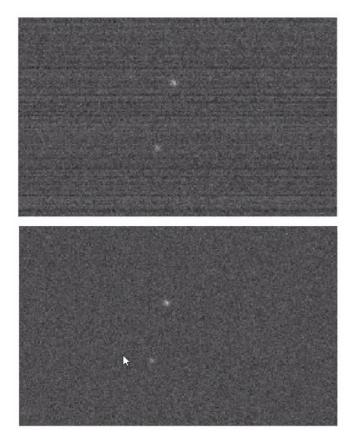
*Figure 15. Comparison of the same image without (top) and with a median signal normalisation. Standard deviation reduced by 8.5 %.*
