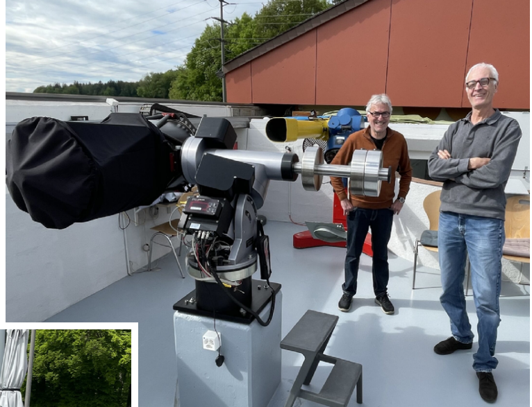
Figure 9. Marco Iten and Stefano Sposetti with the Ritchey Chrétien-Astrograph (Pro RC 360) on a GM4000QCI mount.
