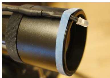
Figure 6.3. Flashing LED connected with the NEXTA device, in this case mounted to the finder telescope, compare Figure 6.1
