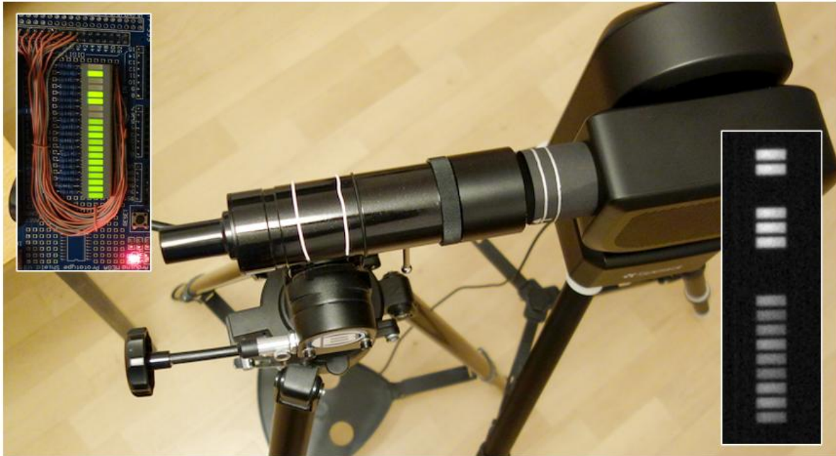
Figure 6.1. Test setup for mapping the NEXTA LED display (image inserted top left) using a finder scope in reverse orientation. The image inserted at the bottom right shows an example from an S50 recording (not showing the actual LED sequence of the image at the top left)
